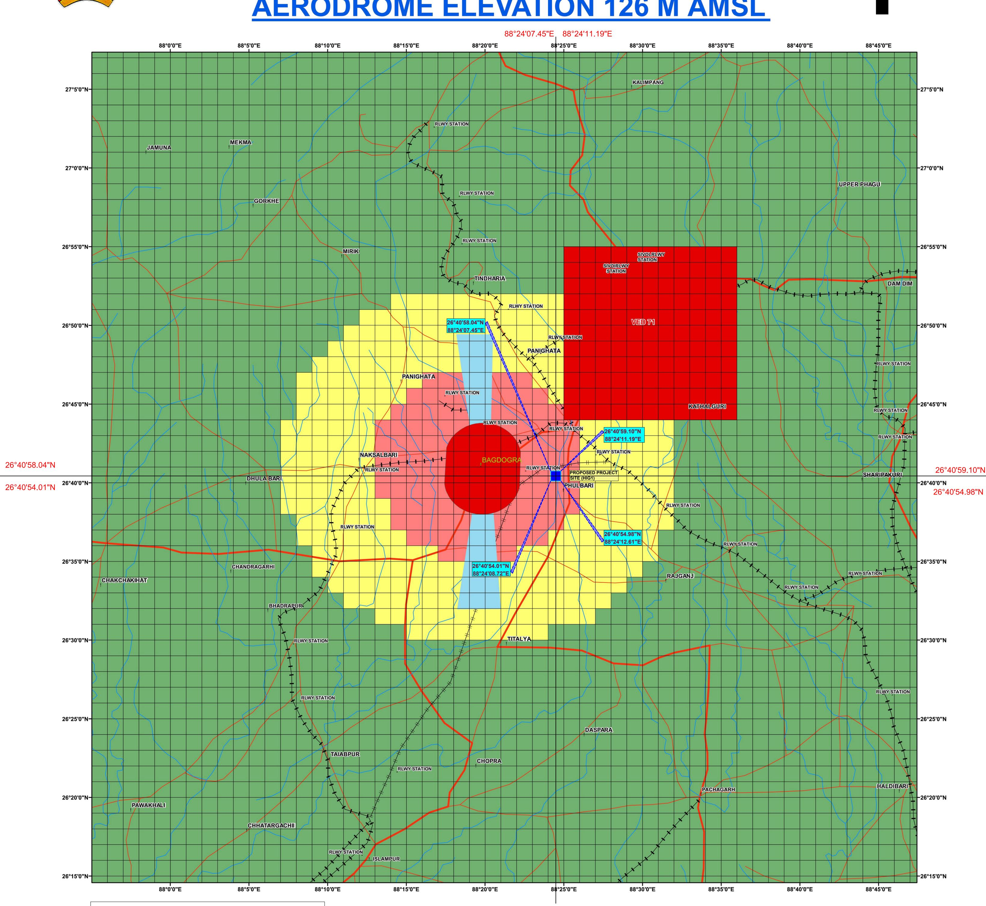
Legend ARP CCZM\_GRID DANGER AREA RAILWAY STATION STREAMS RAILWAY SINGLE LINE ROAD 1ST IMPORTANCE RESTRICTED AREA PROHIBITED AREA ROAD 2ND IMPORTANCE RED: IRRESPECTIVE OF BUILDING HEIGHT, NOC TO BE APPLIED FOR SKY BLUE: NOC EXEMPTED IF TOP ELEVATION IS 140 M AMSL OR BELOW PINK: NOC EXEMPTED IF TOP ELEVATION IS 171 M AMSL OR BELOW YELLOW: NOC EXEMPTED IF TOP ELEVATION IS 246 M AMSL OR BELOW GREEN: NOC EXEMPTED IF TOP ELEVATION IS 276 M AMSL OR BELOW
